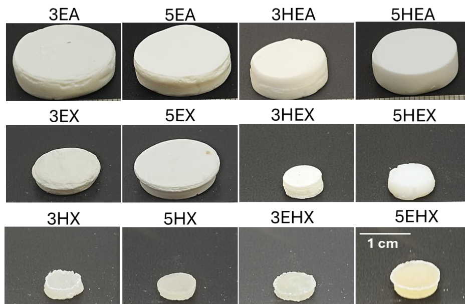
Figure 2. Photos of the dry cellulose materials, aerogels (first row) and xerogels (second and third row). The scale is the same for all samples
