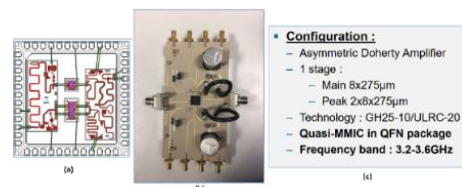
Fig. 1. Layout (a), Demonstration board (b) and Key Characteristics (c) of the realized asymmetric packaged Quasi-MMIC SI-DPA [2].
