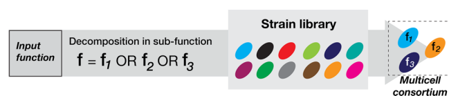
Figure 1. Distribution of a Boolean function within a multicellular consortium. The Boolean function of interest is decomposed as a disjunction ( i.e. , sum) of subfunctions (or clauses). Here, as an example, a given function, f , is decomposed into functions f_1 , f_2 , and f_3 . The strains performing f_1 , f_2 and f_3 are selected from the strain library to assemble a multicellular consortium computing the desired Boolean function.
