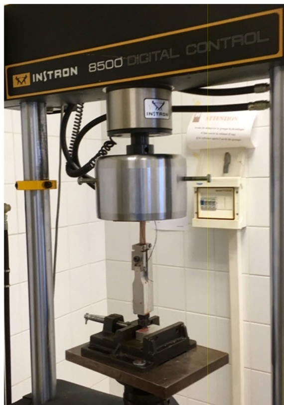
Fig. 4 Loading a hamstring graft on to an Instron® device
