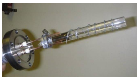
Figure 2c: Rubidium metal sealed in a glass ampoule surrounding by a conductive wire
