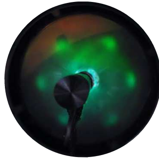
Figure S4: Low-energy electron diffraction (LEED) pattern of the \text{Cr}_{1.6}\text{Te}_2 film taken at 60 eV. It displays hexagonal symmetry thus confirming the observed 2D FFT image as shown in Fig 1. in the main text.
