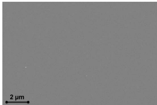
Figure S5: SEM micrograph of the \text{Cr}_{1.6}\text{Te}_2 thin film recorded at a magnification of 20kx. The microstructural surface quality of the \text{Cr}_{1.6}\text{Te}_2 thin film deposited by first harmonic Nd:YAG laser is assessed by scanning electron microscopy. The film grows uniformly over large areas without any
