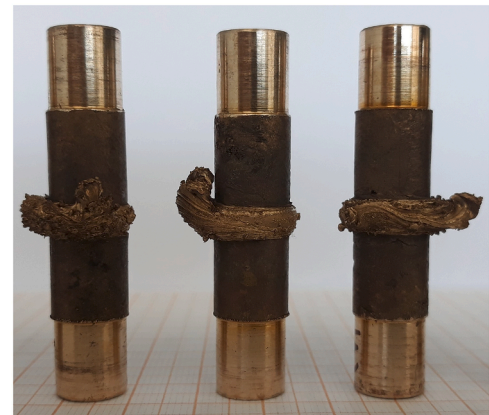
Fig. 4. Cu-11.8Al-0.45Be SMA welded by CDFW and flash characteristics.
