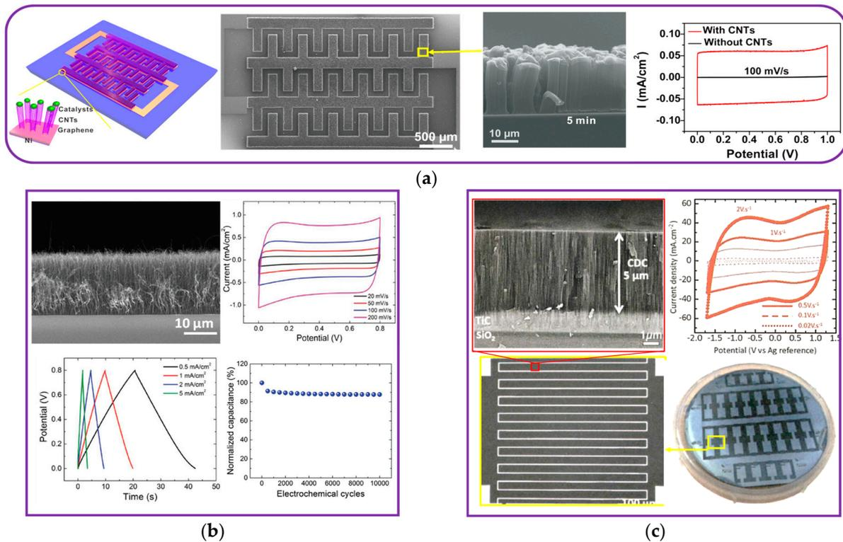
**Figure 7.** Carbon-based electrodes (a) Graphene-CNT grown on a Si substrate. Reproduced with permission from [209]. Copyright © 2024, American Chemical Society. (b) Vertically aligned carbon nanotube (VACNT) forests grown on a silicon wafer. Reproduced with permission from [192]. Copyright (2019), John Wiley & Sons. (c) Carbide-derived carbon (CDC) on a Si wafer. Reproduced with permission from [54]. Copyright (2016), American Association for the Advancement of Science.
