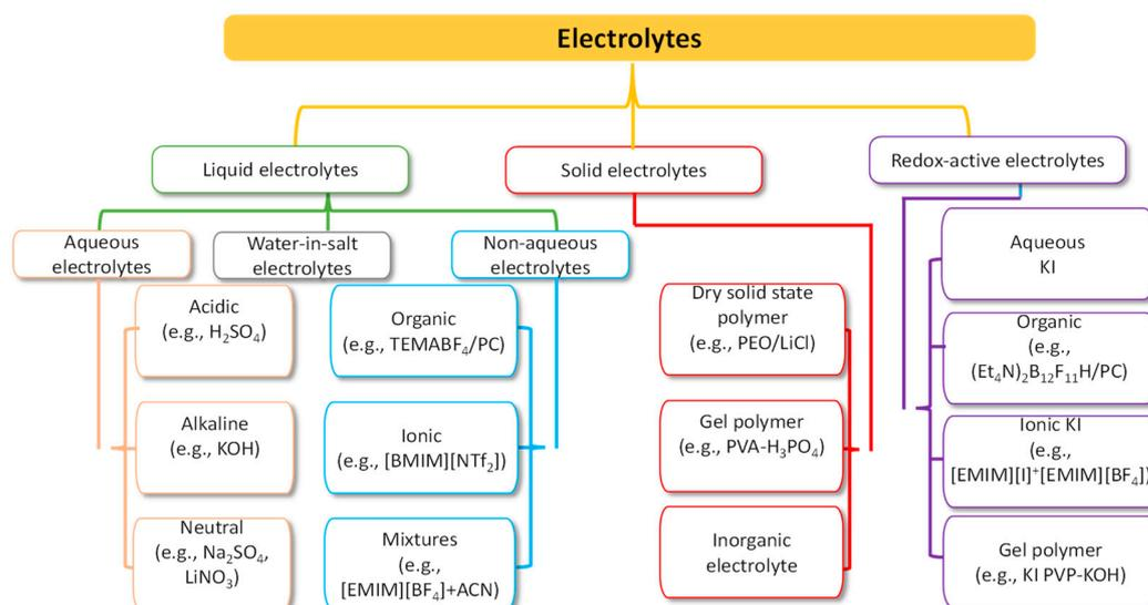
**Figure 12.** Electrolyte classification for MSC applications [465–468].
