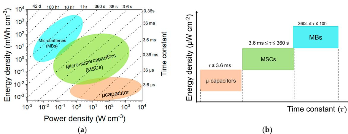
**Figure 1.** Performance of energy storage microdevices. (a) Ragone plot relating energy and power density for the micro-energy storage devices. (b) Energy versus time constant of the various energy storage microdevices.
