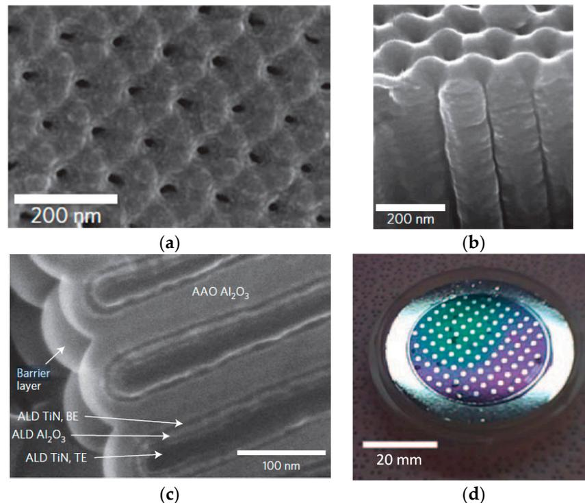
**Figure 5.** MIM nanocapacitor. (a,b) SEM plan-view and cross-section of an AAO MIM structure. (c) The bottom of the tube, showing the AAO barrier layer and three layers corresponding to the TiN bottom electrode (BE),  $\text{Al}_2\text{O}_3$  and the TiN top electrode (TE). (d) Two-inch wafer with nanocapacitors. Reproduced with permission from [67]. Copyright (2009), Springer Nature.
