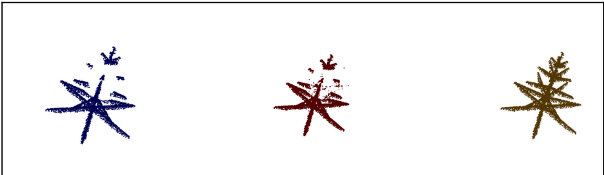
Figure 11: PointTr prediction (red) when the input is the partial point cloud (blue) with the ground truth being the complete point cloud (yellow).
