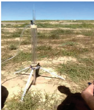
Figure 2. Apparatus of Guelph permeameter
