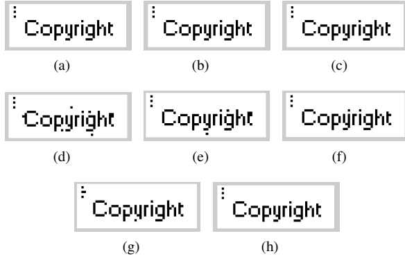
Fig. 5: Extracted watermarks after attacks : (a) Embedded Watermark, (b) Histogram Equalization, (c) Salt & Pepper, (d) JPEG(Q=60), (e) JPEG(Q=65), (f) JPEG(Q=70), (g) JPEG(Q=75), (h) Gaussian Smoothing.
