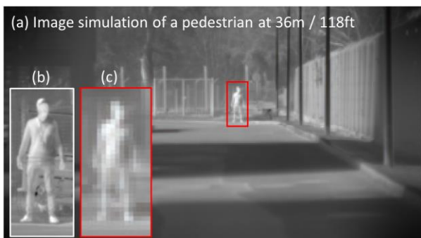
Figure 19: (a) Image simulation of a pedestrian at 36m. Zoomed reference, assumed perfect (b) vs. simulated (c) images.
