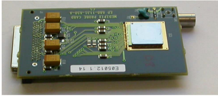
Fig. 4. View of a Medipix2/CdTe detector (1 mm thick) mounted on its front-end electronic board.
