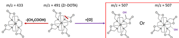
Fig. 7 Simplified degradation pathway for Zr-DOTA radiolysis in water. Compounds framed in red are the major degradation products observed by ESI-MS.
