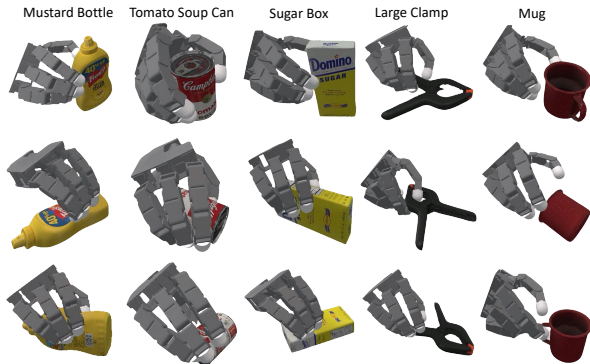
Fig. 2: Motion retargeting results for the Allegro hand and objects under different poses for selected DexYCB videos.
