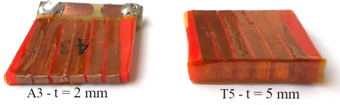
Fig. 3: Photograph of the solenoids characterised in the Figure 2, with ( l = w = 2.4 mm, s_t = 0.5 mm, N = 6 ).
