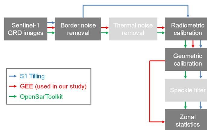
**Figure 11.** Main steps involved in the preprocessing radar signal, according to the algorithm used by FAO (OpenSar toolkit), Google (GEE; Google Earth Engine), and the French national space institute: CNES (S1-Tiling).
