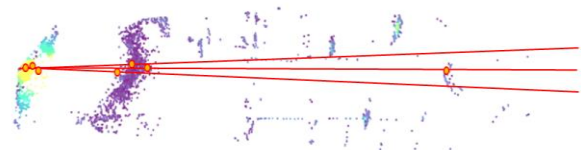
Figure 5: The method of measuring fog points density in the LiDAR point cloud
