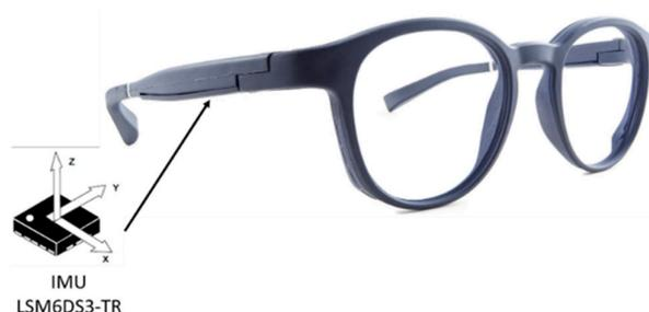
**Figure 1.** Placement of the Inertial Measurement Unit (IMU) in the temple of the smart eyeglasses.
