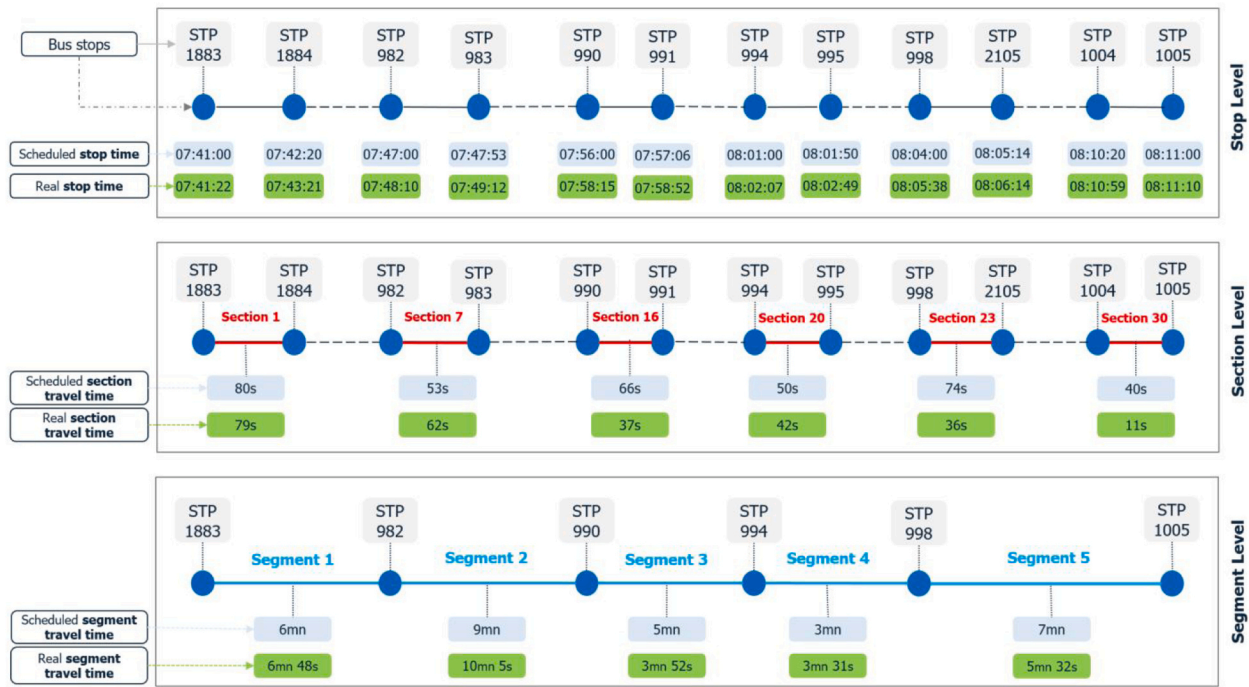
Fig. 4. An illustration of the components of a bus route with stop and travel times.
