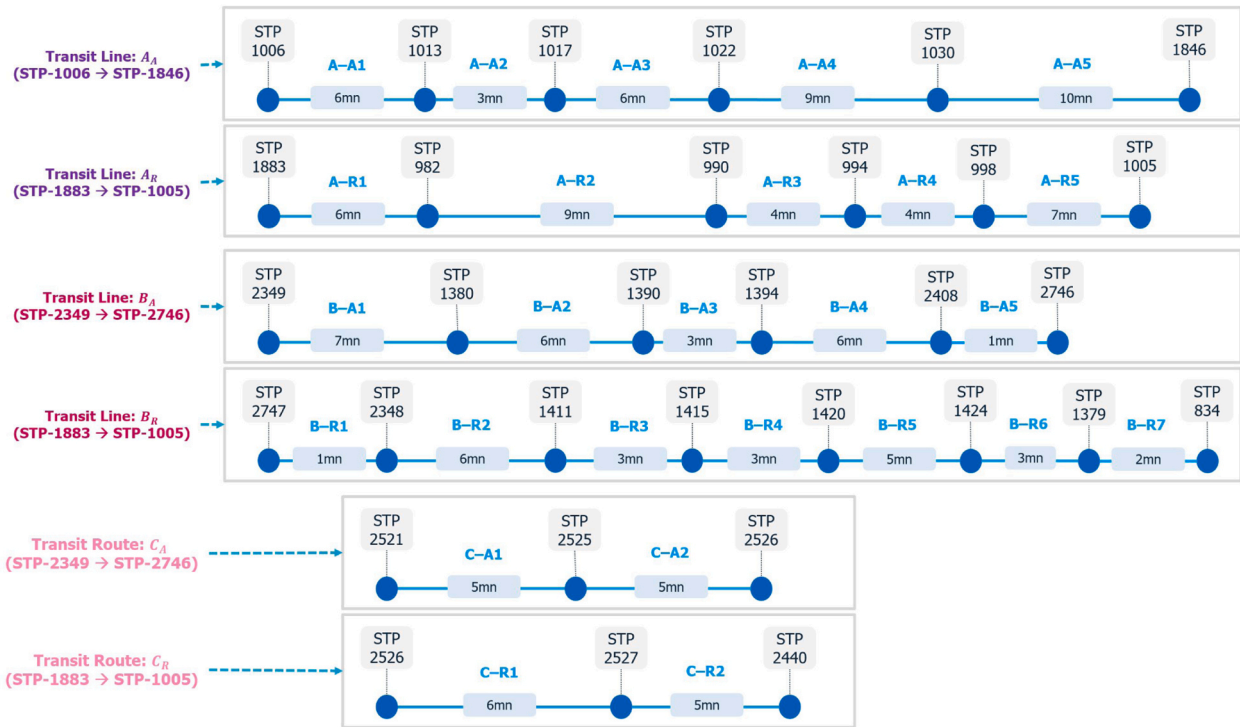
Fig. 11. A detailed illustration of the route segments of the three chosen bus lines. We count, six and three control points per direction for lines A and C respectively; for bus line B, six timing points are defined in the Aller direction, and eight in the Retour direction. The route segment is referenced by: its transit line, its transit route direction (A/R) and its index in the transit route. For instance, A-A2 refers to the second segment of the Aller route of line A.
