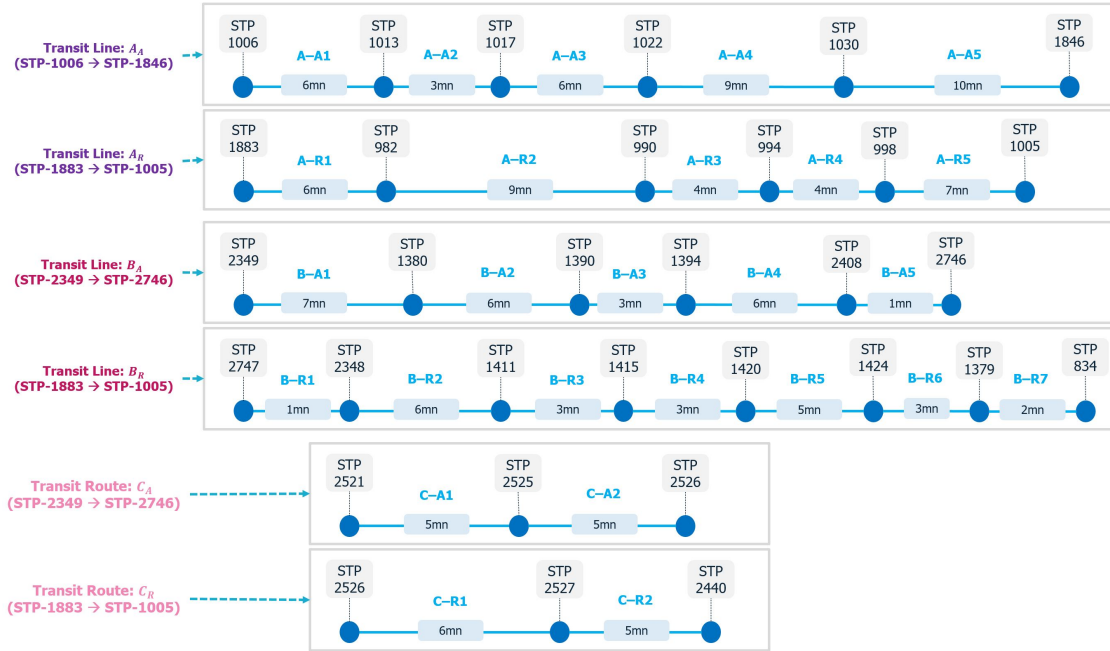
Figure 11: A detailed illustration of the route segments of the three chosen bus lines. We count, six and three control points per direction for lines A and C respectively; for bus line B, six timing points are defined in the Aller direction, and eight in the Retour direction. The route segment is referenced by: its transit line, its transit route direction (A/R) and its index in the transit route. For instance, A-A2 refers to the second segment of the Aller route of line A
