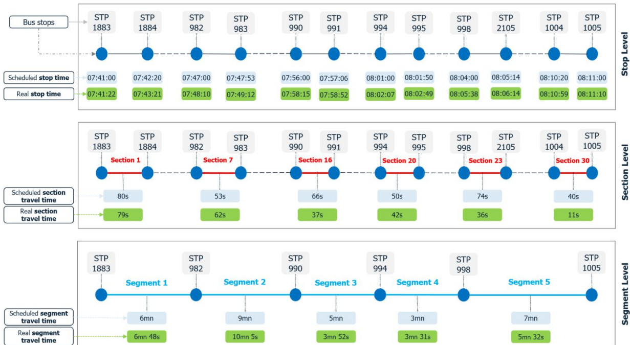
Figure 4: An illustration of the components of a bus route with stop and travel times
