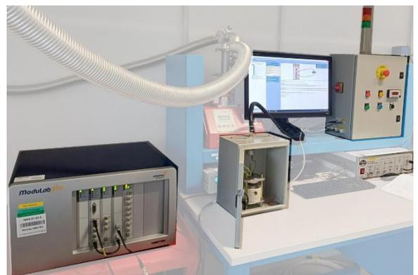
**Figure 4:** DC conductivity test bench. From left to right: ModuLab, sample holder, safety cabinet, voltage amplifier.
