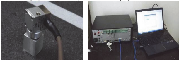
Figure 10. Accelerometers, ADS-2002 system and computer.
