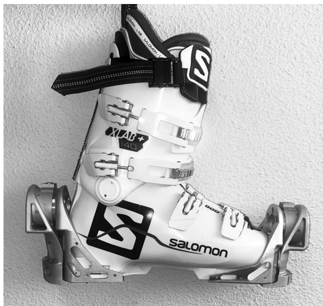
FIGURE 2 Ski-specific force plates. Devices used to collect the primary SRFs data, attached to a pair of standardized boots used during the experiment. More information available in Cross et al., (2021). Each force plate could provide force and moments in three axes (antero-posterior = x, medio-lateral = y, normal = z), but only resultant forces were examined in the present study.
