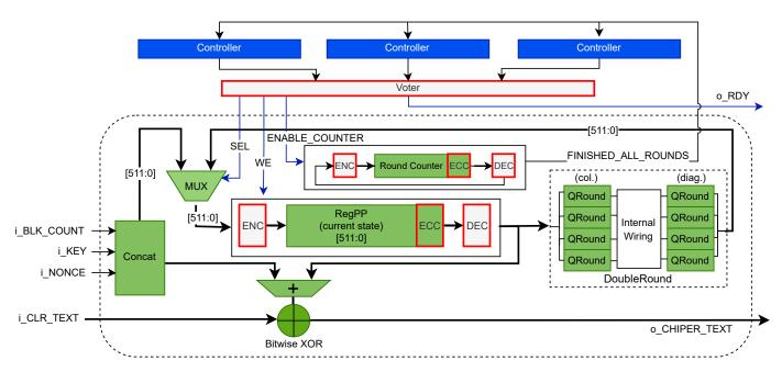
Fig. 1. Block Diagram of the hardened ChaCha20 Accelerator
