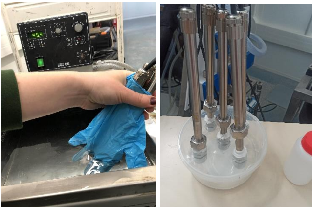
Figure 4. Calibration in (a) temperature and (b) humidity of the sensors
