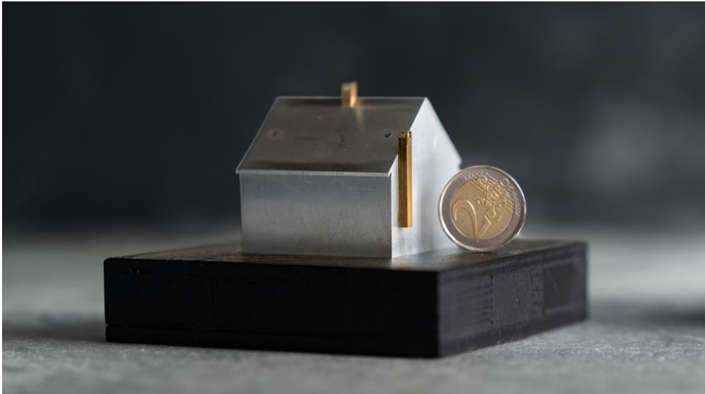
Figure 1: Model house with two stacks. One stack is located at the side of the building and the other stack is placed in the center of the roof.
