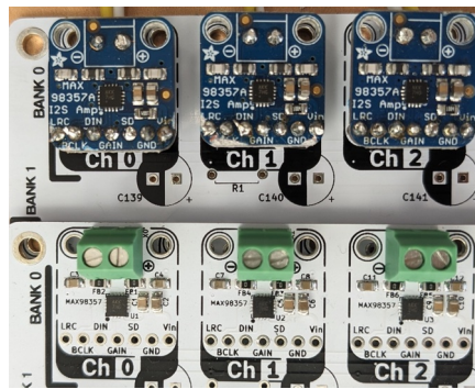
Figure 2. Two Frugal Boards side by side with the two different integration: direct MAX98357A audio codec integration (bottom) or using Adafruit breakout boards (top).
