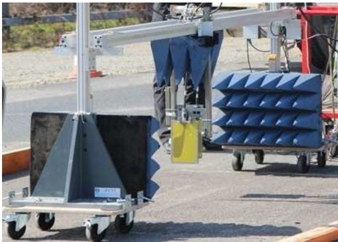
Fig. 10. GPR Data collection at the fatigue carousel using a pair of robot-controlled bistatic antennas over the pavement test area.
