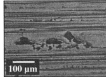
Fig. 7(b) Micro-spalls on the top of longitudinal roughness of large wavelength; AISI 52100 steel; pure rolling; 2.5 GPa,  $5 \times 10^6$  cycles
