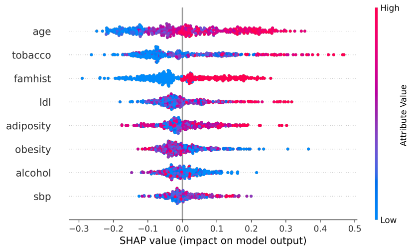
Figure 4: Distribution of KernelSHAP influences for each attribute over the dataset. The attributes are sorted in decreasing mean attribute importance from top to bottom and each dot represents an instance from the dataset, its colour representing the raw value of the attribute. The position on the x-axis represents the contribution of the attribute to the prediction of this individual, and overlapping dots are spread on the y-axis.
