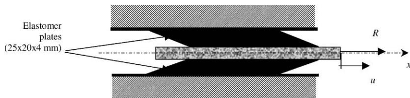
Fig. 10. Elastomer plates subjected to a shear test.
