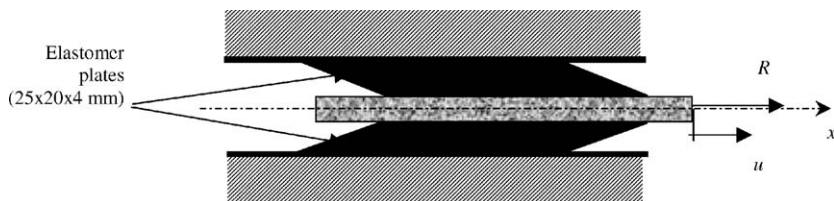
Fig. 10. Elastomer plates subjected to a shear test.
