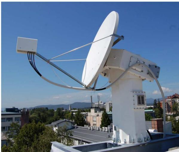
Fig. 2. Antenna and tracking system at JSI flat roof.
