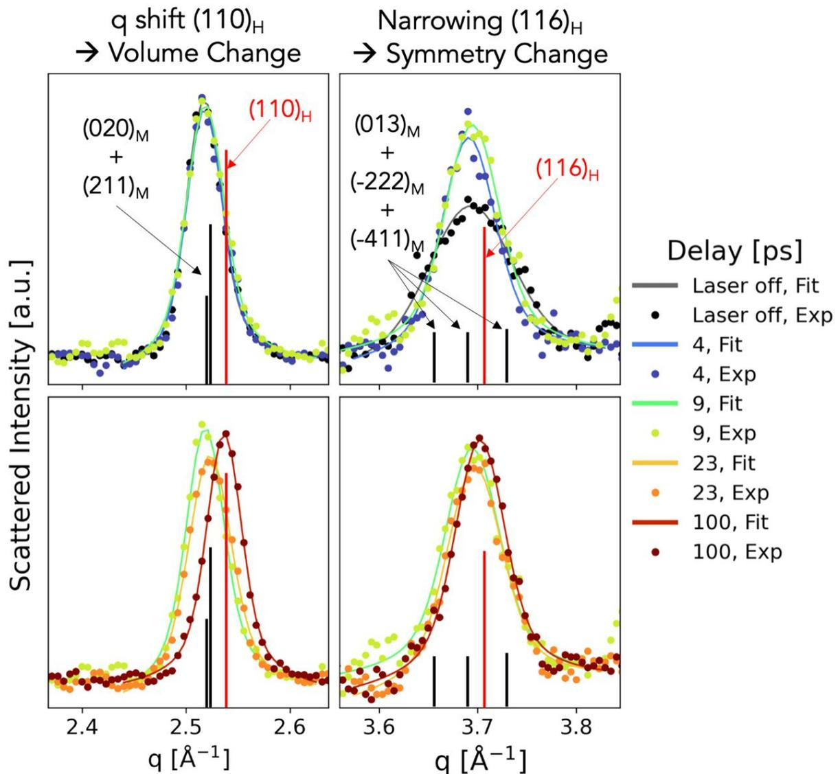
**Extended data Fig.5 | Evidence of different time scale for symmetry and volume change from time-resolved XRD, measured at 10K on the 270 nm film at FemtoMAX.** (Left) Evolution of the  $(110)_H$  Bragg peak for pump-probe delays shorter (top) and longer (bottom) than 9 ps. (Right) Same for the  $(116)_H$  Bragg peak, split into three peaks  $(013)_M$ ,  $(-222)_M$  and  $(-411)_M$  in the initial monoclinic state.
