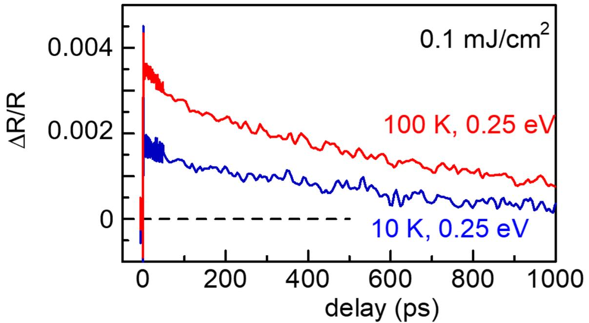
**Extended data Fig.7 | Evidence of long-lived hot electronic states from transient reflectivity data.** Time-resolved reflectivity measured at low pump laser fluence (0.1 mJ/cm<sup>2</sup>, photon energy = 0.89 eV), showing electronic recombination time in the nanosecond range.
