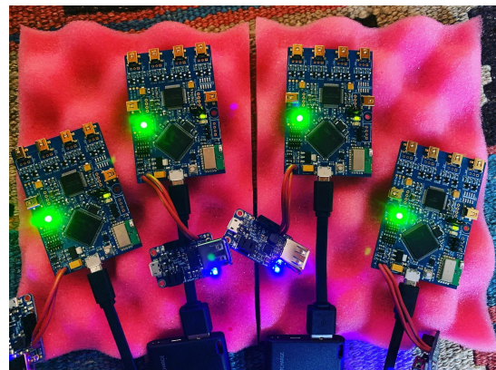
Figure 3. Four EAVI ExG boards
