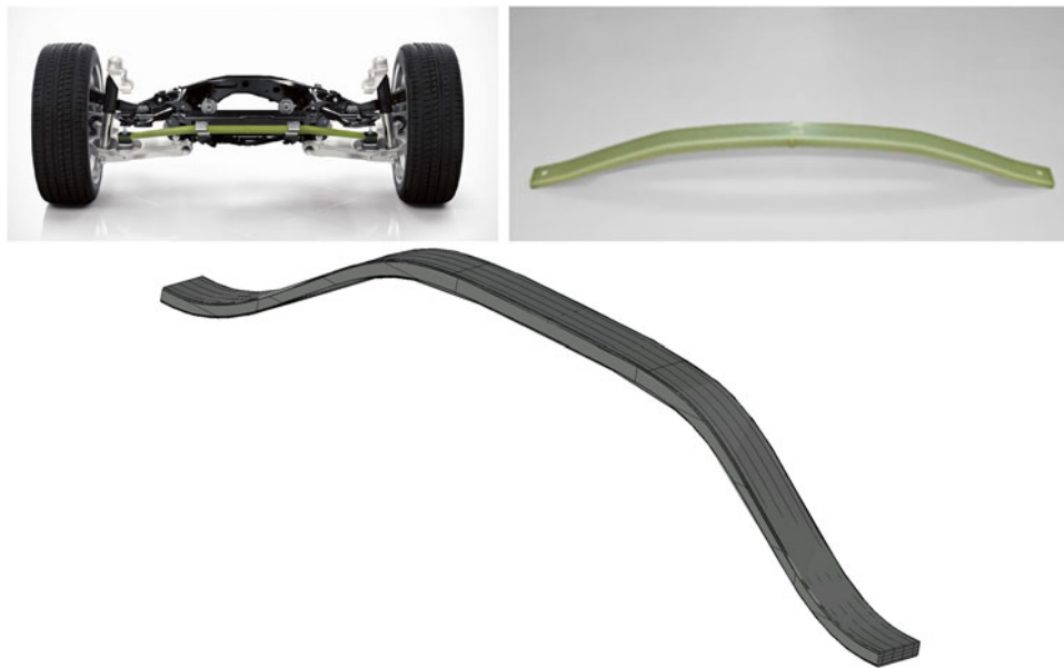
Figure 3. Transverse Rear Leaf springs (top) and assumed geometry (bottom).
