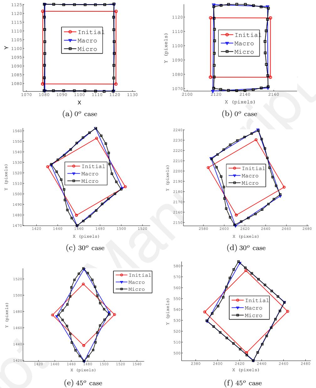
top and right edge of the cell, respectively. When the cell network is aligned with the loading direction ( $0^\circ$ ), cells are mainly loaded in tension along the loading axis. The order 0 parameter is, as expected, predominant for the top edge
