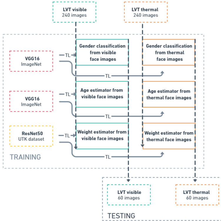
Fig. 3 Transfer learning protocol for soft biometric estimation from visible and thermal images.
