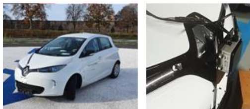
Figure 2 Ego vehicle with the RADAR in front of the logo
