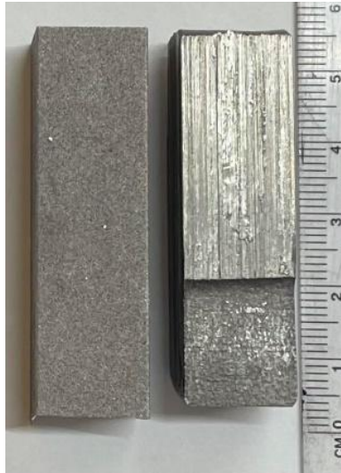
Fig. 2. Illustration of the test samples – LPBF fabricated (left) and ECAP processed (right)
