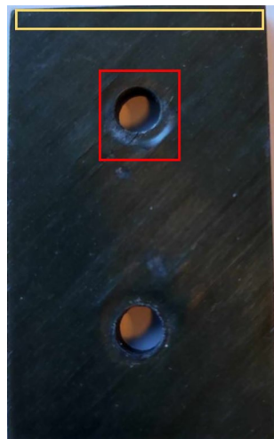
Fig. 9. Photo of the CFRP coupon struck at the ONERA's lightning test facility with the GRIFON generator. The red square corresponds to the area of fastener 1 and is the imaged zone on the CEA's MLSI-XPCI installation. The yellow square corresponds to the undamaged region used to measure the average pristine phase value \phi_0 .
