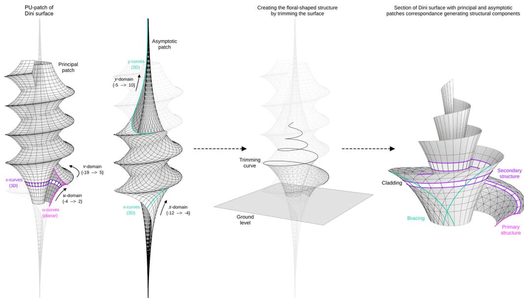
Figure 5: Geometric generation of the floral-shaped structure
