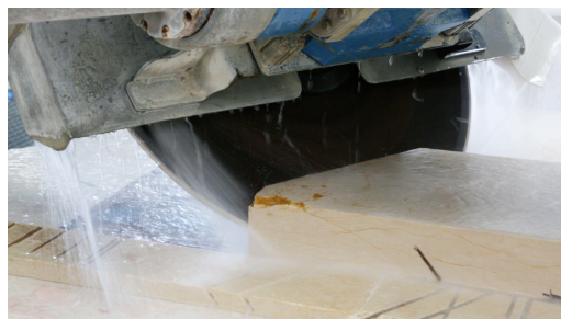
Figure 19: 5 axis cutting machine of edge angles
