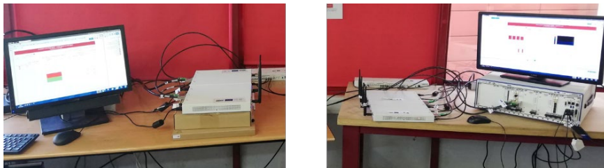
Fig.2. Sounding signal transmitter (left side) and receiver (right side)
