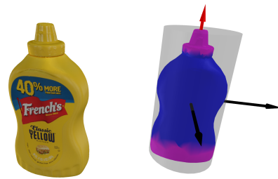
Fig. 2. Mustard bottle from YCB set [17] (left) and a visualization of the corresponding grip selection process (right). Transparent grey volume is the bounding cylinder of the mesh. The red arrow figures the z-axis of the object’s frame. The blue zone illustrates z-values corresponding to a palmar grip, while the magenta zone and outwards correspond to a pinch grip.
