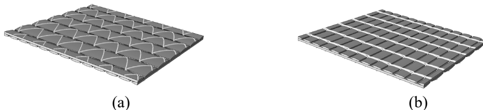
Fig. 2. Geometrical model of biaxial NCF (a) warp yarn view (b) weft yarn view
