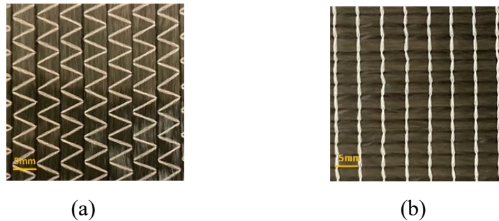
Fig. 1. 0^\circ/90^\circ tricot-stitch biaxial non-crimp fabric architecture (a) warp fiber yarn view with a tricot stitch pattern (b) weft fiber yarn view with a chain stitch pattern
