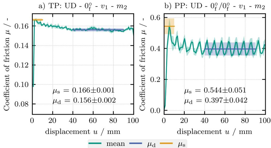
Fig. 3. Schematic illustration of the calculation of the static  $\mu_s$  and dynamic  $\mu_d$  coefficient of friction. The  $\pm$  values give the standard deviation of all tests in the desired range and for the dynamic CoF represent the magnitude of the observed oscillations.
