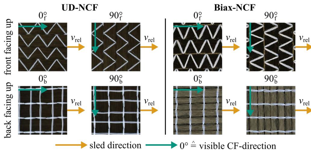
Fig. 2. Naming convention for the inter-ply characterization tests.
