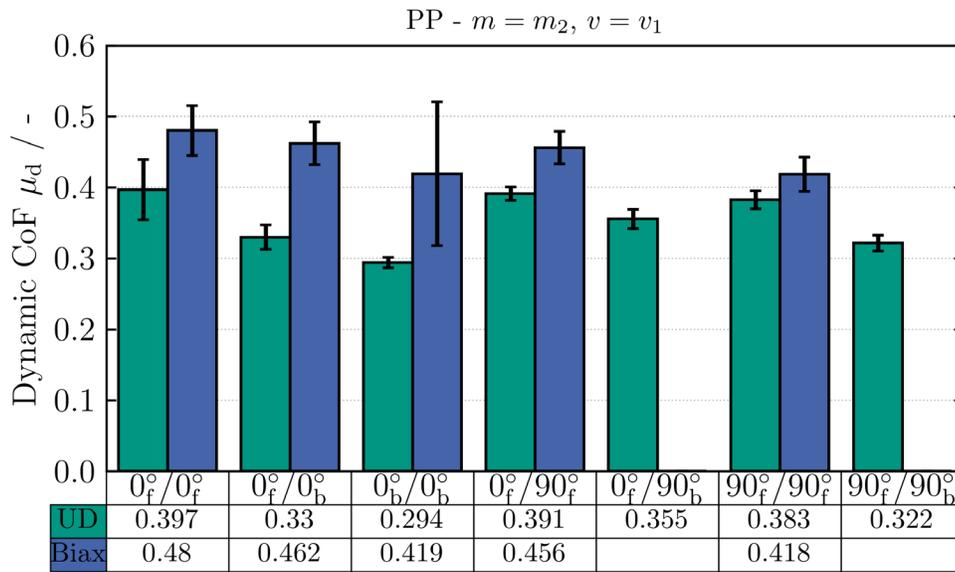
Fig. 6. Influence of the relative interface orientations on the dynamic CoF for the ply-ply behavior with an applied mass of  $m = m_2$  and velocity  $v = v_1$ . The error bars indicate the standard deviation of all tests.
