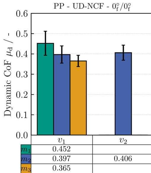
Fig. 5. Influence of the applied mass  $m_i$  and velocity  $v_i$  on the dynamic CoF for the ply-ply behavior of UD-NCF in a  $0_f^\circ/0_f^\circ$ -configuration. The error bars indicate the standard deviation of all tests.
