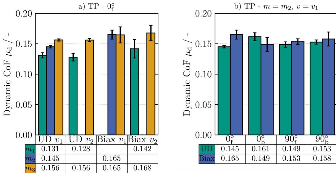
Fig. 4. Experimental results of the tool-ply (TP) dynamic CoF | (a) Influence of the applied mass  $m_i$  and velocity  $v_i$  in a  $0_f^\circ$ -configuration for both materials; (b) Influence of the relative interface orientations with an applied mass of  $m = m_2$  and velocity  $v = v_1$ . The error bars indicate the standard deviation of all tests.
