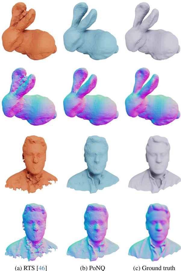
Figure 9. Learning-based results for PoNQ. Optimization-based results for Reach For the Spheres [46]. Note that both methods rely on the same input, here a 32^3 SDF grid. RTS can either miss thin structures (bottom rows) or fill thin voids (top rows).
